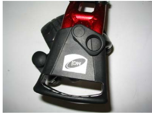
2. When unlocked the front wheel assembly can swivel 360 degrees
