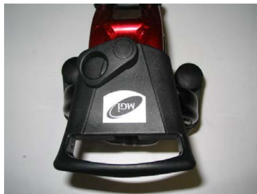
3. When locked the front wheel sits behind the front handle
